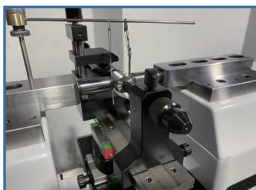
Thread measurement plug gauge
