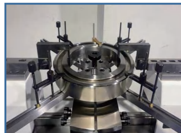
Large ring gauge for calibration
