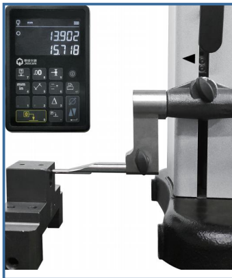
Hole position measurement, intuitive and simple
