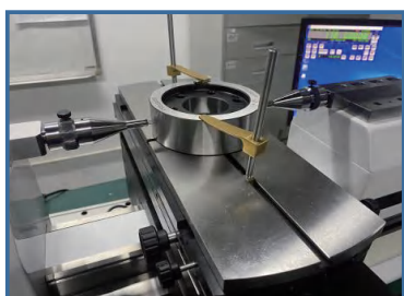
Smooth surface measurement plug gauge
