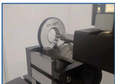
Tapered thread ring gauge for calibration
