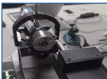
Tapered thread plug gauge for calibration
